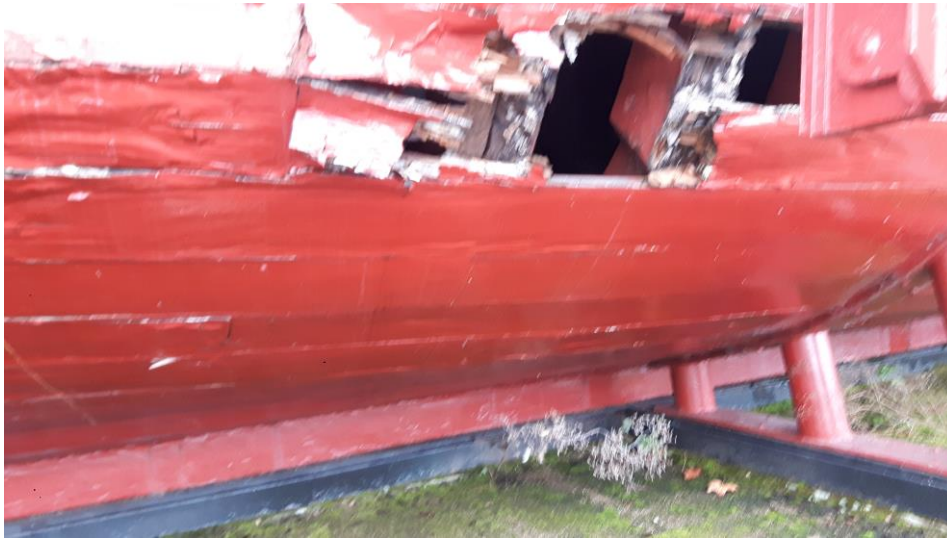
Rotten planking port side
